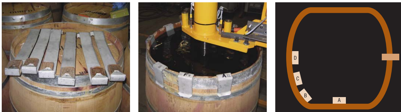
Figure 1. Brettanomyces/Dekkera infected sliced blocks clipped onto surface-sterilised metal holders (A), which in turn were clipped onto the side of the barrel (B) for treatment with HPU applied through the open head of a 225L barrel of water. Positions of slice blocks in the barrel (C) for HPHW and MPHw treatment (Block D is affixed to a stave directly opposite the bung-hole).
